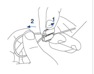
4) Position wire between the first and second baffle and the ninth and tenth baffle
