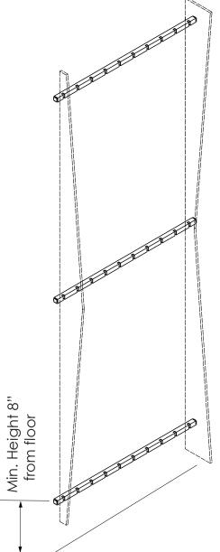
Appy Liquid Nails General Purpose to inside of extrusion prior to fixing the blades.
