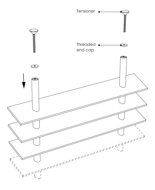
8) Compress louvers with threaded end cap & screw out tensioner as required.
